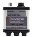
The eMorpho is a single-input multichannel analyser, designed to work with all scintillators.
