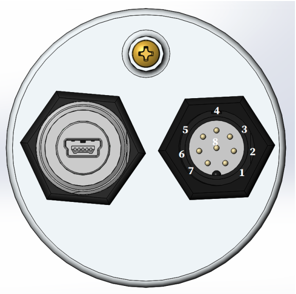
Fig. 31: Pin numbers on the EN3P8 (8-pin GPIO) connector. The connectors and pinouts are the same for the PMT-2000 and the SiPM-2000.
