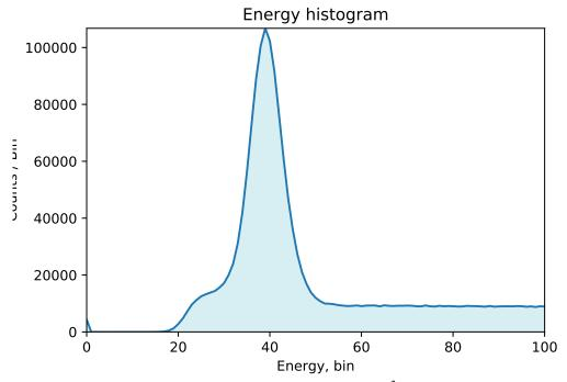
Cs-137 spectrum on a 50x50mm high-quality NaI(Tl) crystal, 2.4x2.4cm<sup>2</sup> Broadcom SiPM array. The energy resolution is 6.56%fwhm at 662keV. Gain and operating voltage were adjusted for a maximum measurable energy of 3.2MeV. Notice in the bottom panel that the spectrum cleanly extends to below 22keV.
